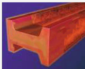
Beam partially descaled
